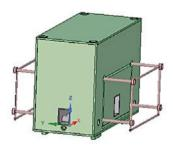
gitudinal axis. The remaining internal space of the case is occupied with cells made of gas-protecting clothe and filled with helium, ensuring buoyancy. The gas volume is sufficient for weight compensation of aircraft structure, units and assemblies, pilot and an additional load of about 200 kg.
