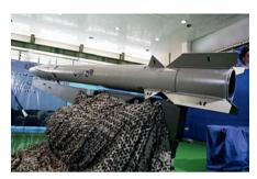
Initially the missile range was just 200 km and its precision was very moderate, however, the missile stayed guided until the very end. The missile's precision and range have been improved and increased gradually with further development of Iranian industry. After the last modification, the Fateh-110 missiles have a range of about 300 km and warhead weight of 448 kg.
